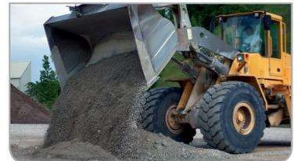
After mixing for a few minutes with **RE-CON ZERO**, concrete is transformed into granular material which may be discharged on the ground and, once cured, used as aggregate in concrete. **RE-CON ZERO** works with all types of concrete.
